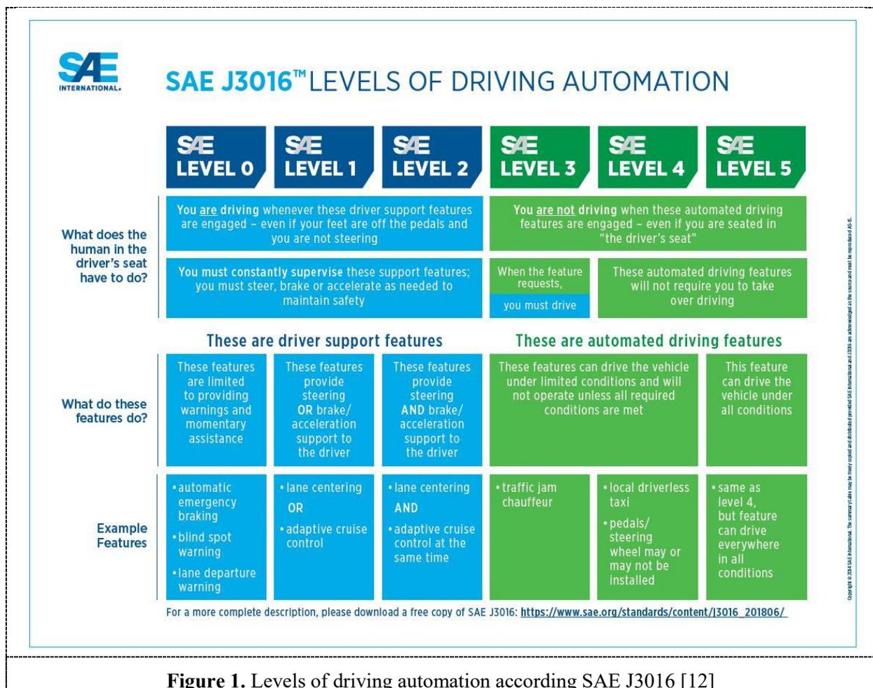
**Figure 1.** Levels of driving automation according SAE J3016 [12]
