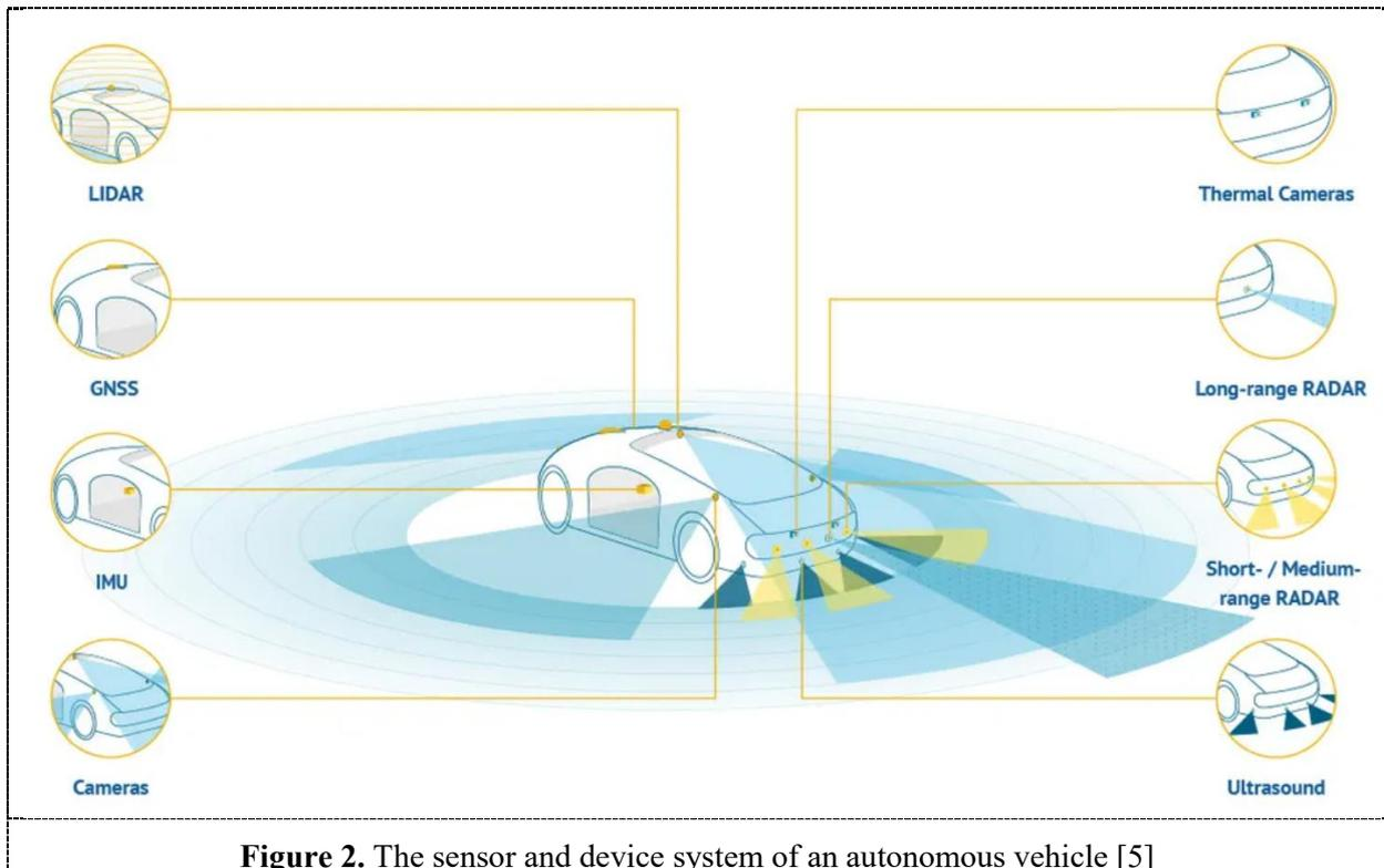
**Figure 2.** The sensor and device system of an autonomous vehicle [5]
